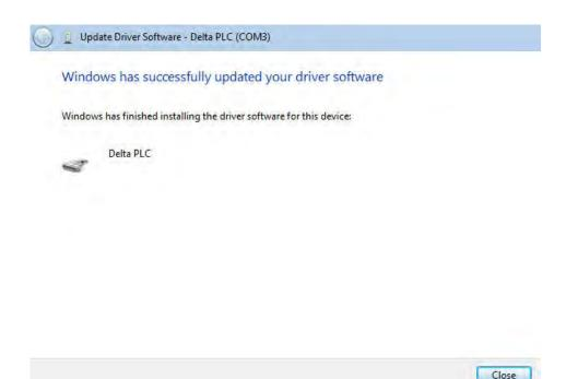
(8) Open the Device Manager window again. If the name of the Delta USB device appears under Ports (COM & LPT), the installation of the driver is successful. The operating system assigns a communication port number to the USB device.
