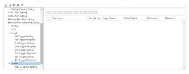
The system for the DVP-ES3/EX3/SV3/SX3 Series module supports data transmission between the CPU module and other CPU modules or devices through a socket as well as through TCP and UDP protocols. You can set up connections through both protocols in the **TCP** and **UDP** setting pages.
