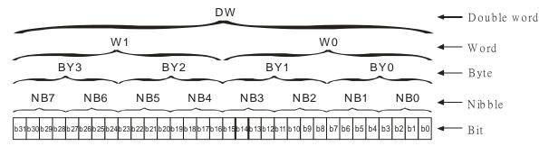
The PLC uses four types of values to execute the operation according to different control purposes.
