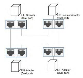
ES Series PLC CPU does NOT support DLR. If you need to join a DLR network, it is suggested to use a switch with DLR function, DVS-103I02C-DLR.
