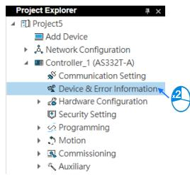
(2) The **Device & Error Information** window appears. Click **to refresh the log and click** to clear the error log in the window and the error log in the CPU module.
