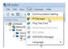
The IP Manager can be the BOOTP/DHCP Server, receiving IP address requests from devices. The IP Manager window is shown below.
