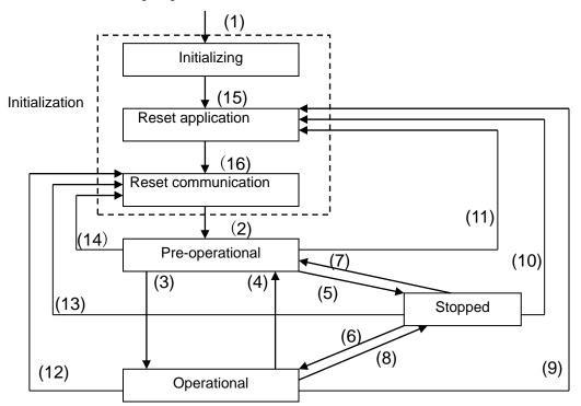
(1) After power is supplied, the device automatically enters the initialization state.
