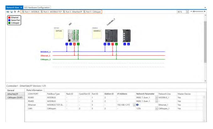
These types of parameters are used to create a data exchange table for the built-in communication ports of the DVP-ES3/EX3/SV3/SX3 series models. The DVP-ES3/EX3/SV3/SX3 series models can act as masters for exchanging data with remote devices acting as slaves.
