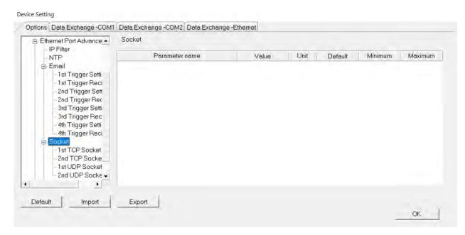
The system for the DVP-ES3 Series module supports data transmission between the CPU module and other CPU modules or devices through a socket as well as through TCP and UDP protocols. You can set up four connections in each of the four groups. Select the **Socket Function Enable** checkbox and then select settings in the **TCP** and **UDP** setting pages.
