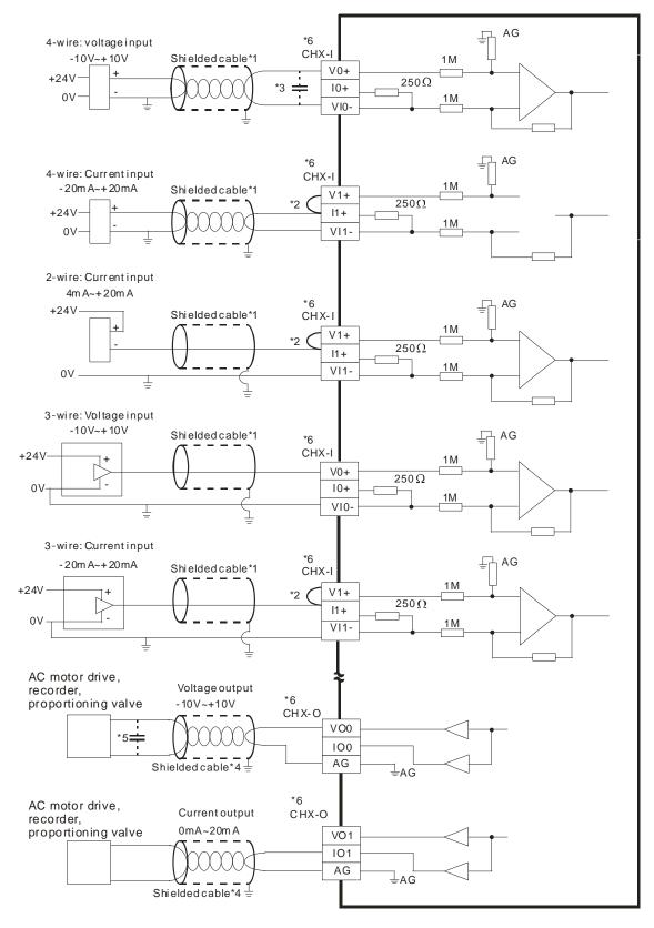
\*1. Use shielded cables to isolate the analog input signal cable from other power cables.
