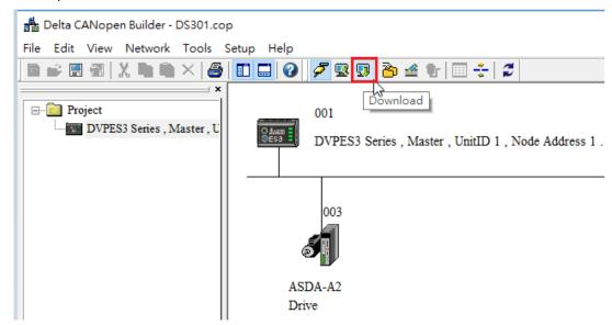
Note: you must reboot the DVP-ES3 Series PLC to enable the downloaded parameters.
