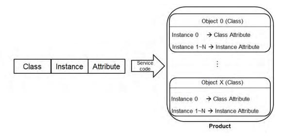
The supported EtherNet/IP objects are listed in the following table. Refer to Section 9.8.2 for the data type definitions. Refer to Section 9.8.3~9.8.19 for object contents. You can use explicit messages to read and write Objects. DVP-ES3/EX3/SV3/SX3 Series PLC acts as a Scanner, you can use EIPRW instruction to read and write Objects. Refer to DVP-ES3/EX3/SV3/SX3 Series Programming Manual for more details on EIPRW instruction (API2208).
