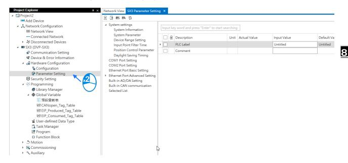
Delta Electronics provides you with specific configuration tools for some CPU modules. You can add extension modules to the right side of the DVP-ES3/EX3 Series CPU module. And for DVP-SV3/SX3 series, you can install extension modules on its both sides (left and right). There are Configurations (for CPU modules) and Parameter Setting (for CPU parameters) under the Hardware Configuration. And the built-in CAN communication setting allows you to change the CAN port work mode.
