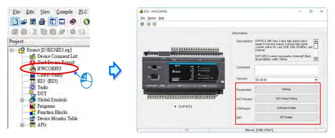
Delta Electronics provides you with specific configuration tools for some CPU modules. You can add extension modules to the right side of the DVP-ES3 Series CPU module. The system configuration area displays the present system configuration. When you modify the configuration in the system configuration area, the information in the information list updates.
